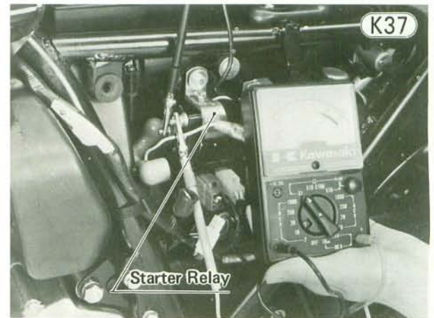
Starter Relay Contact Test
